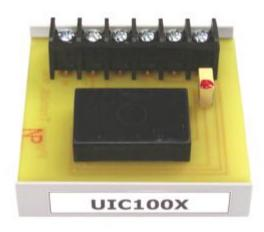
The UIC100X is designed to allow UVR, VR and XR series voltage regulators to be controlled by an analog or digital signal from devices such as genset controllers, power factor controllers, PLCs, and any other device which can input a 0 to 10vdc or +/- 10vdc signal into it.
